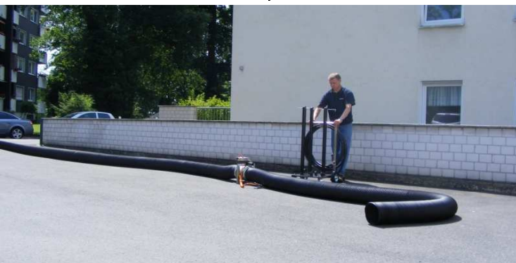
AIRJET on chassis with 15m and 10m air supply hose
